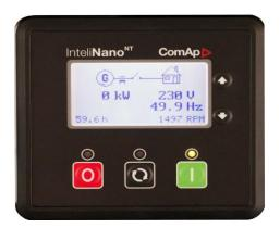
Powergen Pacific Standard Control Panel uses micro processing technique integrating digital, intelligent and network techniques which can carry out functions including auto start/stop, data measure, alarming. The controller uses LCD display. It can be widely used in all types of generator automatic control system for compact structure, advanced circuits, simple connections and high reliability. USB interface and ECU support CAN J1939.
